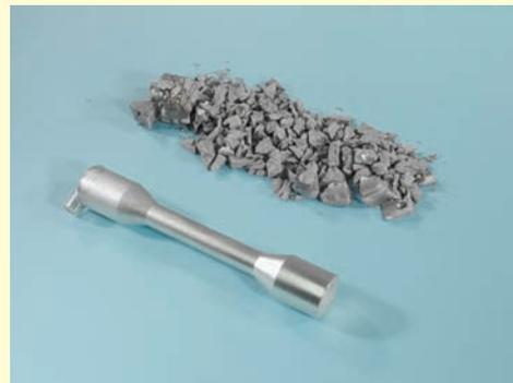
Specimen of white tin (left). Another specimen disintegrated upon transforming to gray tin (right) after it was cooled to and held at a temperature below 13.2°C for an extended period of time. (Photograph courtesy of Professor Bill Plumbridge, Department of Materials Engineering, The Open University, Milton Keynes, England.)
